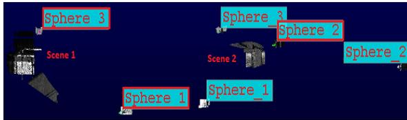
**Figure 2:** Both scenes and all spheres form two views before registration. Red boxes show the spheres from the first view.
